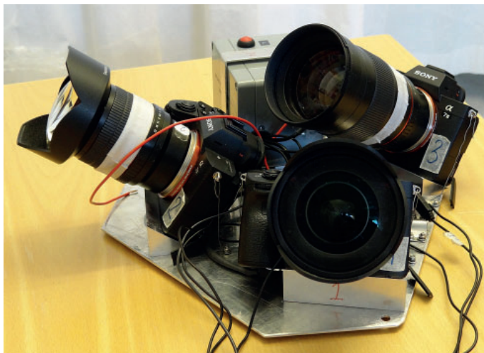
Fig 2.1.2 Det nybyggda instrumentet kallat SONC - Stratospheric Observations of Noctilucent Clouds (Foto: Peter Dalin)
